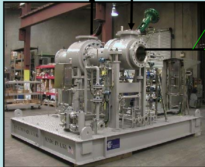
TURBOEXPANDER" / "ELECTRIC GENERATOR" (T/G) SYSTEM
